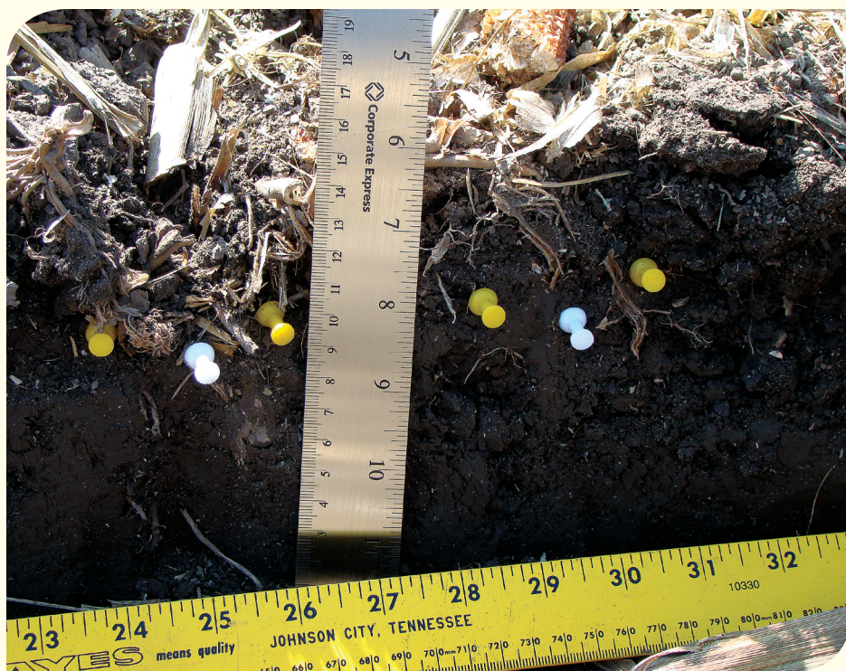
A single pass with a shallow vertical tillage tool disturbed about 40% of soil surface, according to University of Wisconsin Discovery Farms research. The white pins mark coulter blade depth of a Summers Supercoulter Plus vertical tillage machine. The colored pins mark soil disturbance width.
