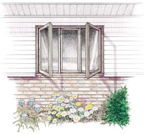
For some bizarre reason, with casement windows (windows that crank open like doors) and some custom-built storm doors, the swing direction is determined exactly the opposite as it is for doors. When you're trying to find out the swing direction of a door, pretend you're strad-
